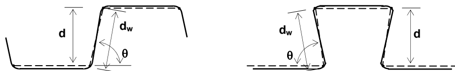
Figure 11.2b - Idealized section for sheet profile
